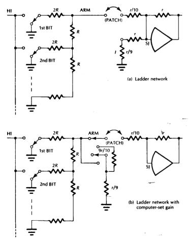
Figure 5 - Binary-weighted-ladder summing networks
