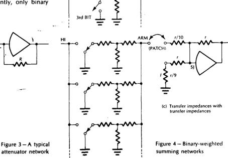
Figure 4 illustrates some binary-weighted attenuator
