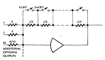
Figure 7 – Simple version of a summing amplifier with switched gain
