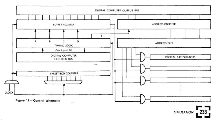
The control signals for both the MANUAL and AUTO-MATIC modes are compared in figure 13. Note that in either mode the last pulse resets all of the flip-flops in the control logic, and in the AUTOMATIC mode it also sends a signal back to the computer to show that the coefficient has been set. Appendix A contains a schematic diagram of a typical digital attenuator card.
