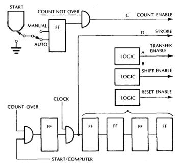
Figure 12 – Simplified timing logic
